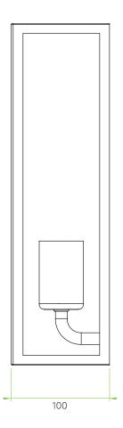
Recess in wall for Terminal Block 60x60x30mm
