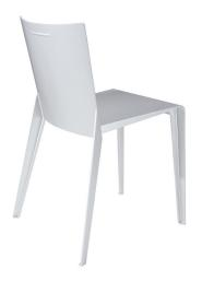
Alfa was born from the union of just two pieces: one is the back, which continues into the rear legs; the other is the seat that extends into the front legs. Both pieces are in composite polyester resin composite, material with added fibreglass. Alfa can be glossy and matt lacquered.
