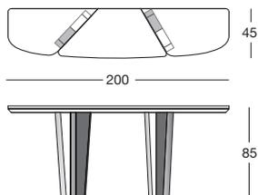
Console consisting of 2 trapezoidal legs and a shaped and sectioned top made of different materials.
